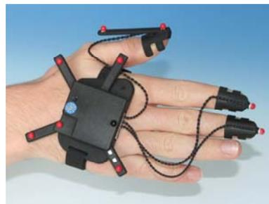
Figure 1: Finger tracking hardware.
